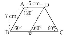
$$\overline{BE} = \overline{AD} = 5 \text{ cm}, \angle B = 180^\circ - 120^\circ = 60^\circ$$
